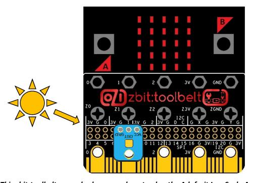
This zbit:toolbelt example shows you how to plug the Adafruit Log-Scale Analog Light Sensor onto zbit:toolbelt and use it to display the ambient light level as a bar graph on your micro:bit
