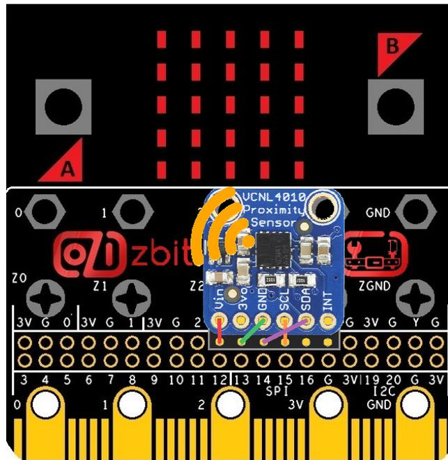
*This zbit:toolbelt example shows you how to plug the Adafruit VCNL4010 Proximity Sensor into zbit:toolbelt and use it to display the proximity of a object as a bar graph on your micro:bit display and make a Proximity Controlled Musical Instrument!*
