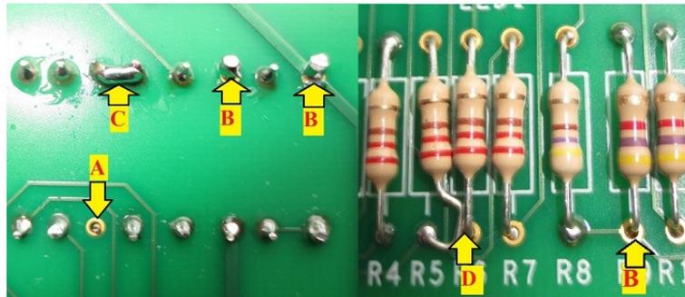
Most of these could be rectified just using the soldering iron, pliers and/or cutters, but for some large solder blobs I used a solder-sucker...
